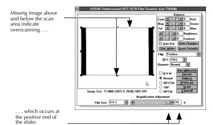
You determine the "optimal" setting for your images. To ensure that as many pixels of the imager as possible are used for you images, your image should fill the scanning area vertically. This will typically occur with the slider in the middle (nominal) range of the scanner either at, or within a few percentage points either way, of the center of the slider.
